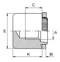
Female thread A = M3,5Height K = 9.0Min thread length C = 4.0Outer diameter E = 10.0Plate thickness = 1.7 to 1.9
